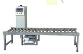
Very accurate weighing system (For E – Type)
